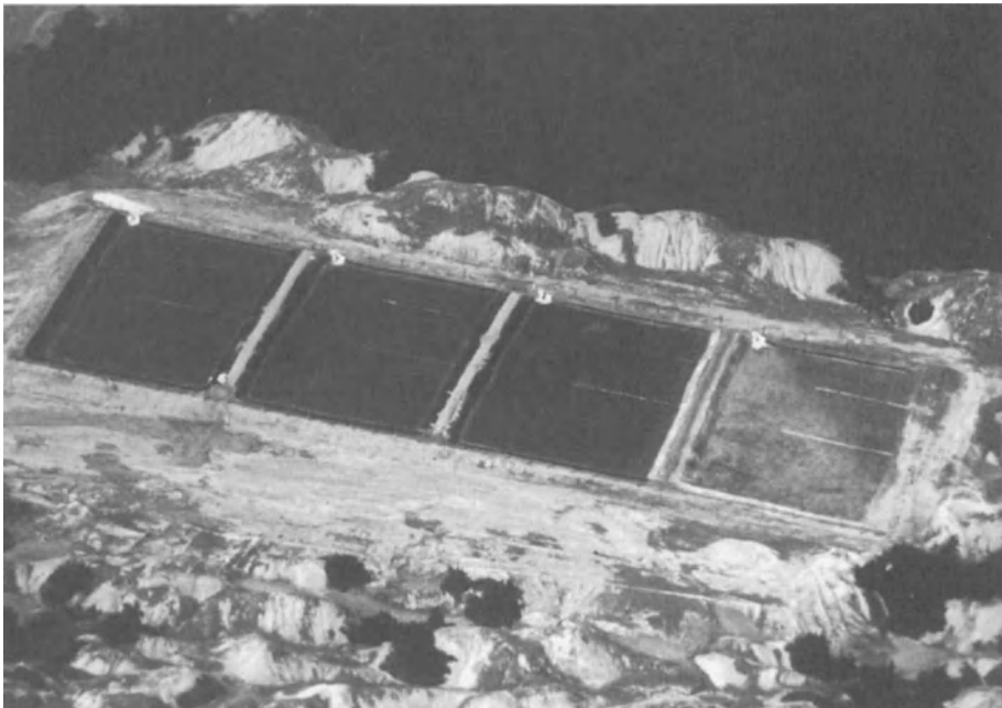
Fig. 1. Aerial view of demonstration reclamation site and the pyritic overburden from strip mining at Ottawa, Illinois. Plot 4 is on the left : the untreated Plot 1 is on the right . Note the Parshall flumes in the upper left-hand corner of each plot
